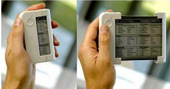
Philips RADIUS rollable display prototype. Is the new Japanese consortium taking a different path?
